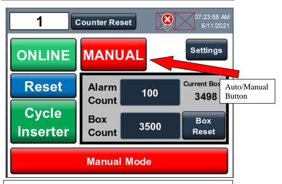
The Auto/Manual Button: If the Inserter is in Manual Mode the inserter will be in fault and the Cycle Button is the only thing that will signal the Inserter. The Inserter must be is Auto Mode to run.
