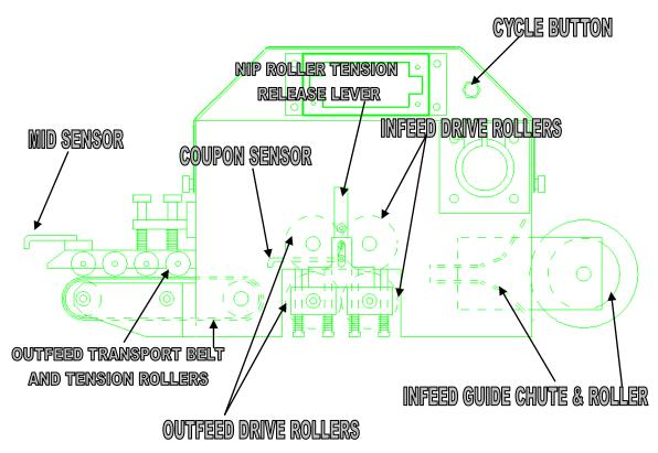
This diagram of the 1600 SRV Inserter shows the location of some common parts.
