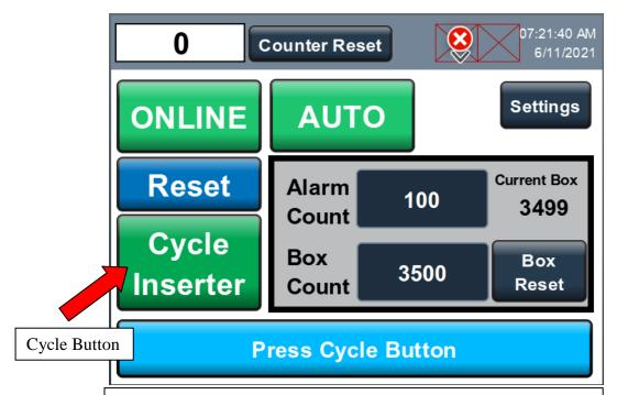
After Pressing the Offline/Online Button. The Servo drives are enabled and the inserter is ready. Feed the inserts into the Infeed rollers and press the Cycle Button.
