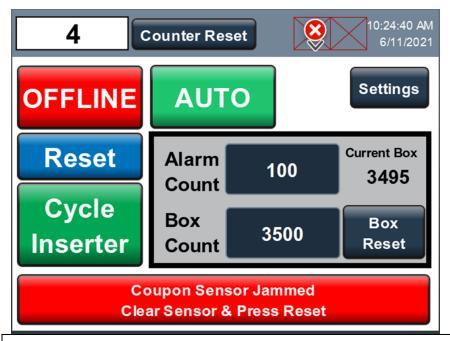
Coupon Sensor Jammed: This fault occurs when an insert/coupon gets stuck under the Coupon Sensor. To clear this fault clean out the inserter. Then press the Reset Button.
