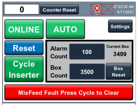
If at anytime the Inserter gets a signal to insert and no insert is seen by the Coupon Sensor, the Inserter goes into the Misfeed Fault. Loading inserts into the machine and pressing the Cycle button will clear the fault.
