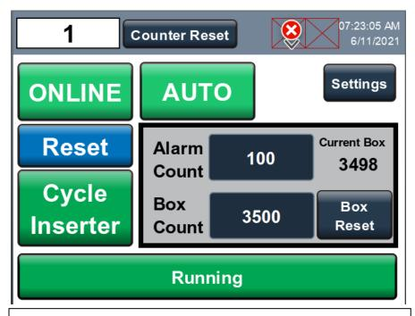
After the inserter sees one insert run through, it will then enter a Running State. The Green light will be on.
